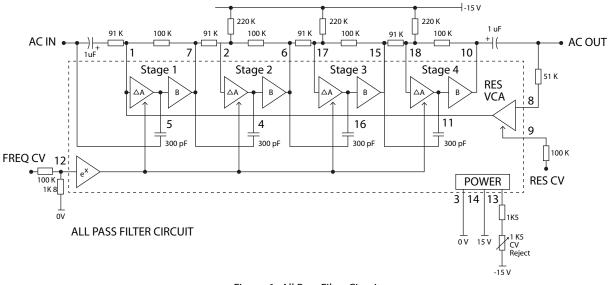
Figure 6. All Pass Filter Circuit
