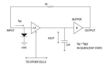
The quiescent output voltage of each buffer,  $V_{ODC}$ , should be set to 0.46 $V_{CC}$  for lowest control voltage feed-through and maximum peak-to-peak output signal, so the  $R_F$  in Figure 2 can be calculated as follows:
