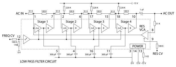
Figure 3. Low Pass Filter Circuit
